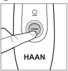
Press ON/OFF button. Wait 20 seconds for unit to heat up. Unit may vibrate while heating.
